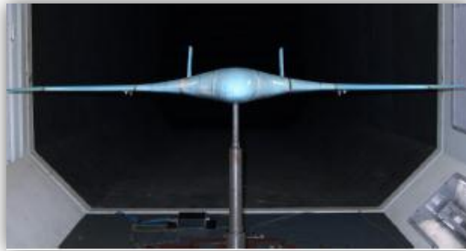
Figure 4. Half-scale model installed in the 7 by 5 ft wind tunnel in Sydney
