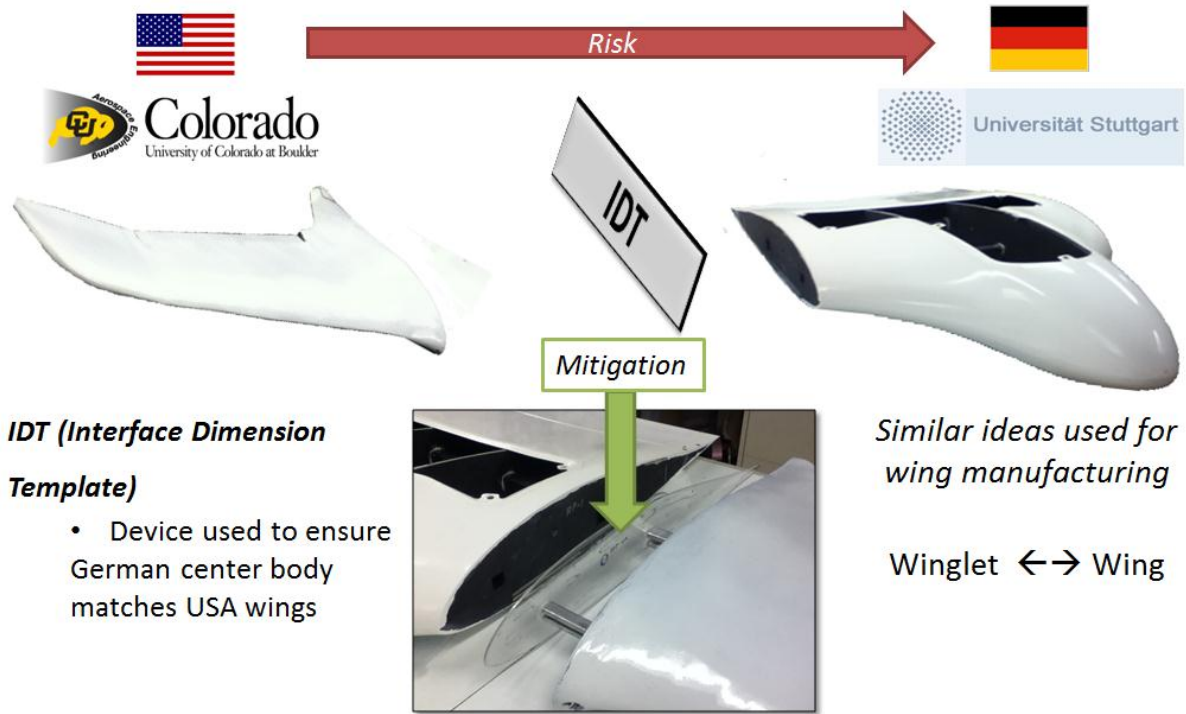
Figure 8. The Interface Dimension Template Guaranteed Wing & Center Body Integration.
